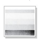
Using the Self Test Print shown above, you can make adjustments to the printer settings such as media width and media thickness (printhead pressure). The location of these two adjustments is explained in section 3.h and also shown on the labels on the printer's
